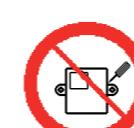
Do not open the Control Unit box for any reason, especially when the engine is running or the key is in the ignition, to avoid irreparable damage.
