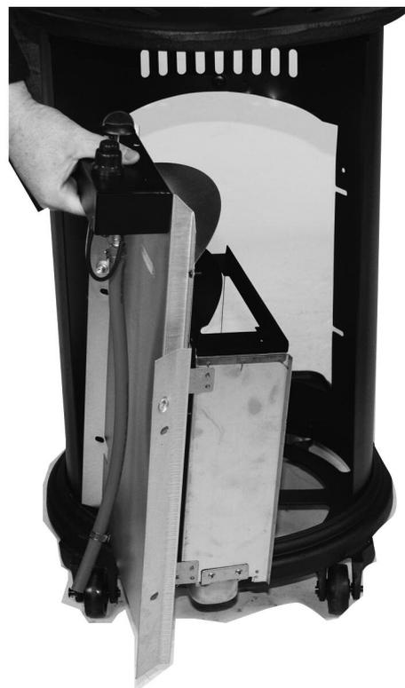
Carefully install the new burner chamber and reassemble in place.
