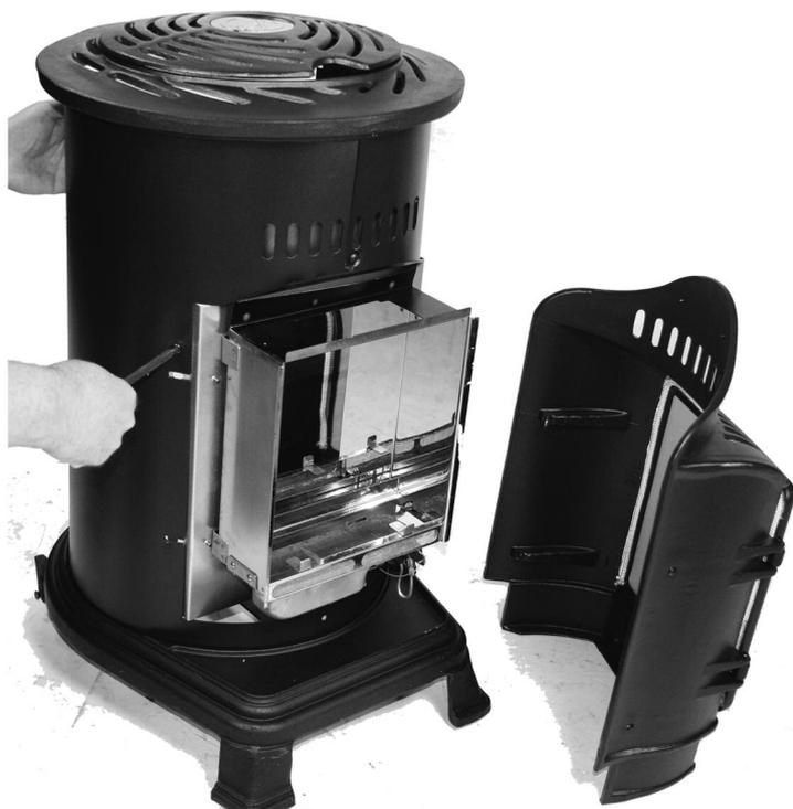
After removing the front cast section unscrew the 4 philips screws which will release the burner chamber from the Provence frame.
